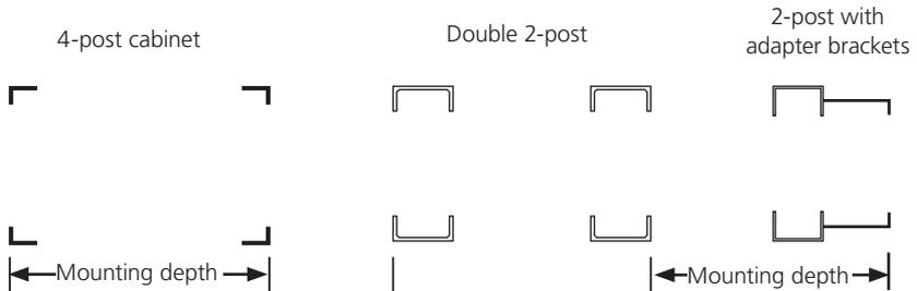
Figure 1. Mounting depth measurements.
