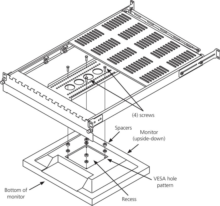
Figure 6. Attaching the monitor.
