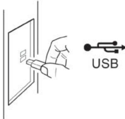
9. Insert the DMS cartridge firmly into the USB cradle. Avoid 'slapping' the cartridge into place. The green and red indicator lights should illuminate. The DMS cartridge will then be detected by the operating system.
