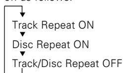
The REP indicator lights up when repeat play is turned on. The track number blinks in the display when track repeat is on. The disc number blinks in the display when disc repeat is on.
