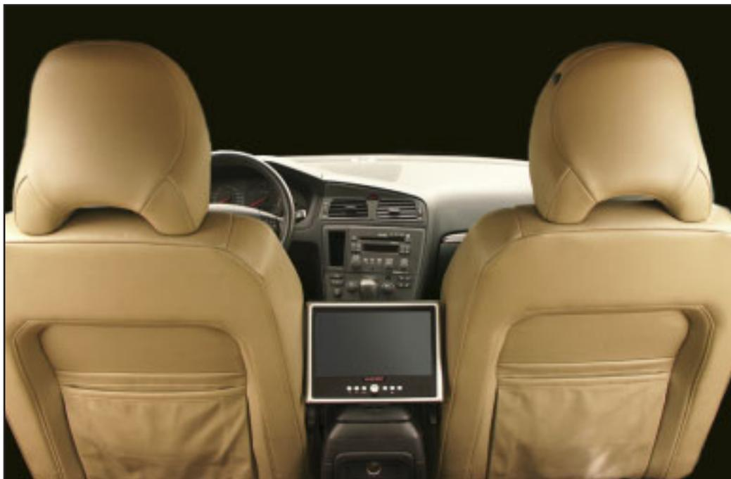
Brodit offers an easy-to-use system for mounting multimedia monitors in the vehicle. It is based on a car specific mount with a monitor mount. The monitor will be placed between the front seats, giving the back seat passengers a perfect view.
