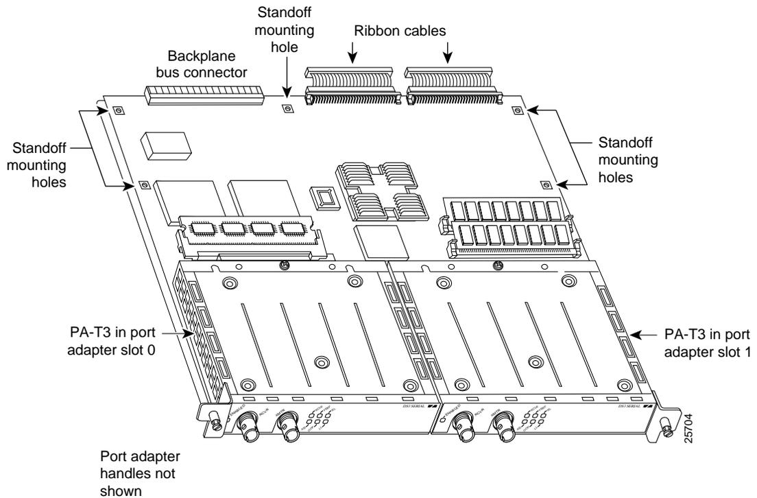
**Note** Port adapters have a handle attached, but this handle is not shown to allow a full view of detail on each port adapter's faceplate.
