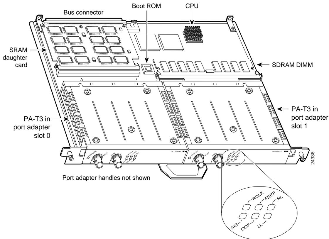
Depending on the circumstances, you might need to install a new port adapter on a VIP2 motherboard or replace a failed port adapter in the field. In either case, you need a number 1 Phillips screwdriver, an antistatic mat on which you can place the removed interface processor, and an antistatic container in which you can place a failed port adapter for shipment back to the factory.
