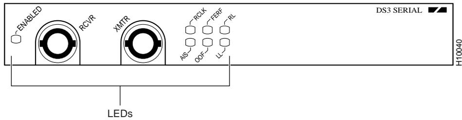
The PA-2T3 has one status LED and six uplink port status LEDs (RCLK, FERF, OOF, AIS, RL, and LL) for each serial PA-T3 port. (See Figure 2-2.)
