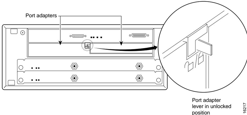
**Step 3** Grasp the handle on the port adapter and pull the port adapter from the router midplane, about halfway out of its slot. If you are removing a blank port adapter, pull the blank port adapter completely out of the chassis slot.
