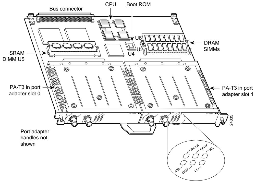
**Note** Port adapters have a handle attached, but this handle is not shown to allow a full view of detail on each port adapter's faceplate.
