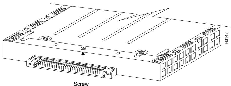
**Step 5** Remove the screw that secures the port adapter (or blank port adapter).
