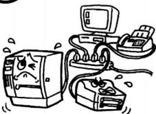
If the machines share the same outlet with any other electrical appliances which consume large amounts of power, the voltage will fluctuate widely each time these appliances operate. Be sure to provide an exclusive outlet for the machine as this may cause **fire** or **electric shock**.
