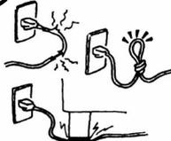
Do not scratch, damage or modify the power cords. Also, do not place heavy objects on, pull on, or excessively bend the cords, as this may cause **fire** or **electrical shock**.
