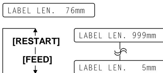
**[FEED]** key: Pressing the **[FEED]** key once causes a -1 mm change, down to 5 mm.
