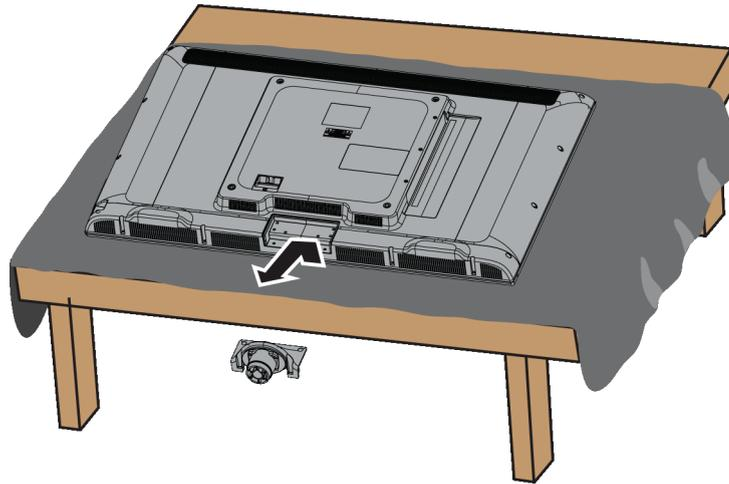
4 Attach the wall-mount bracket to your TV using the mounting holes on the back of your TV. See the instructions that came with the wall-mount bracket for information about how to correctly hang your TV.
