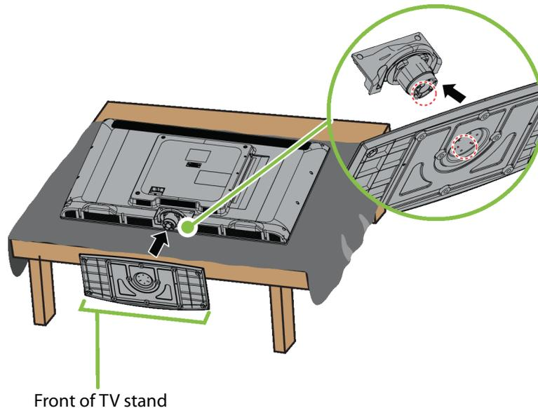
3 Secure the stand with the six provided screws.
