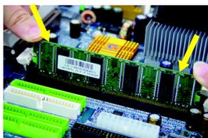
3. Close the plastic clip at both edges of the DIMM slots to lock the DIMM module. Reverse the installation steps when you wish to remove the DIMM module.
