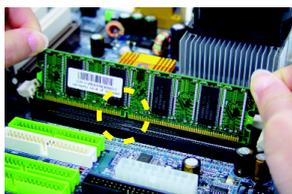
2. Insert the DIMM memory module vertically into the DIMM slot. Then push it down.
