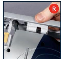
**Note.** For accurate work it is necessary to do a practise cut first. Check the cut and reset the angle until the correct cut is achieved.
