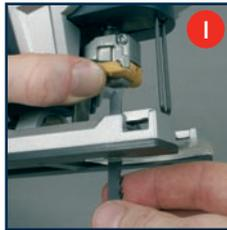
With the blade change control (17) in its uppermost position, remove the blade by pulling it downwards towards the base of the jigsaw.
