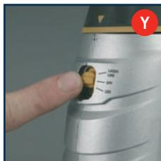
To use the laser wait until you have commenced cutting then set the laser light on/off switch (12) to the on position.
