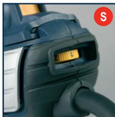
Rotate the dial (8), located at the back of the jigsaw to set the blade speed (fig S).
