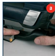
Switch on the jigsaw and allow the blade to reach maximum speed.
