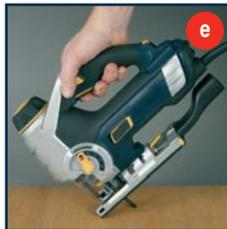
When cutting tight curves, reduce the speed of the saw.
