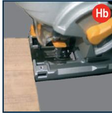
2. With a blade fitted move the variable speed dial (8) to number 3 (low speed).
