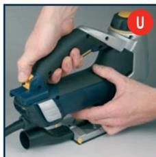
To refit the handle, slide the handle into position with the handle locating pin (11) in the slot at the back of the jigsaw housing. Push it fully forward until the handle release catch (10) locks positively into position (fig V).
