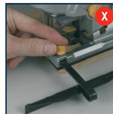
Slide the fence to the required cut width and tighten the locking knob to secure the fence in position (fig X).
