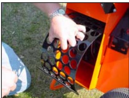
The Discharge Screen is easily removable making the change from screen to screen a breeze.
