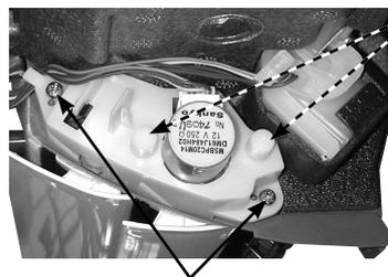
Screws of the horizontal vane motor
