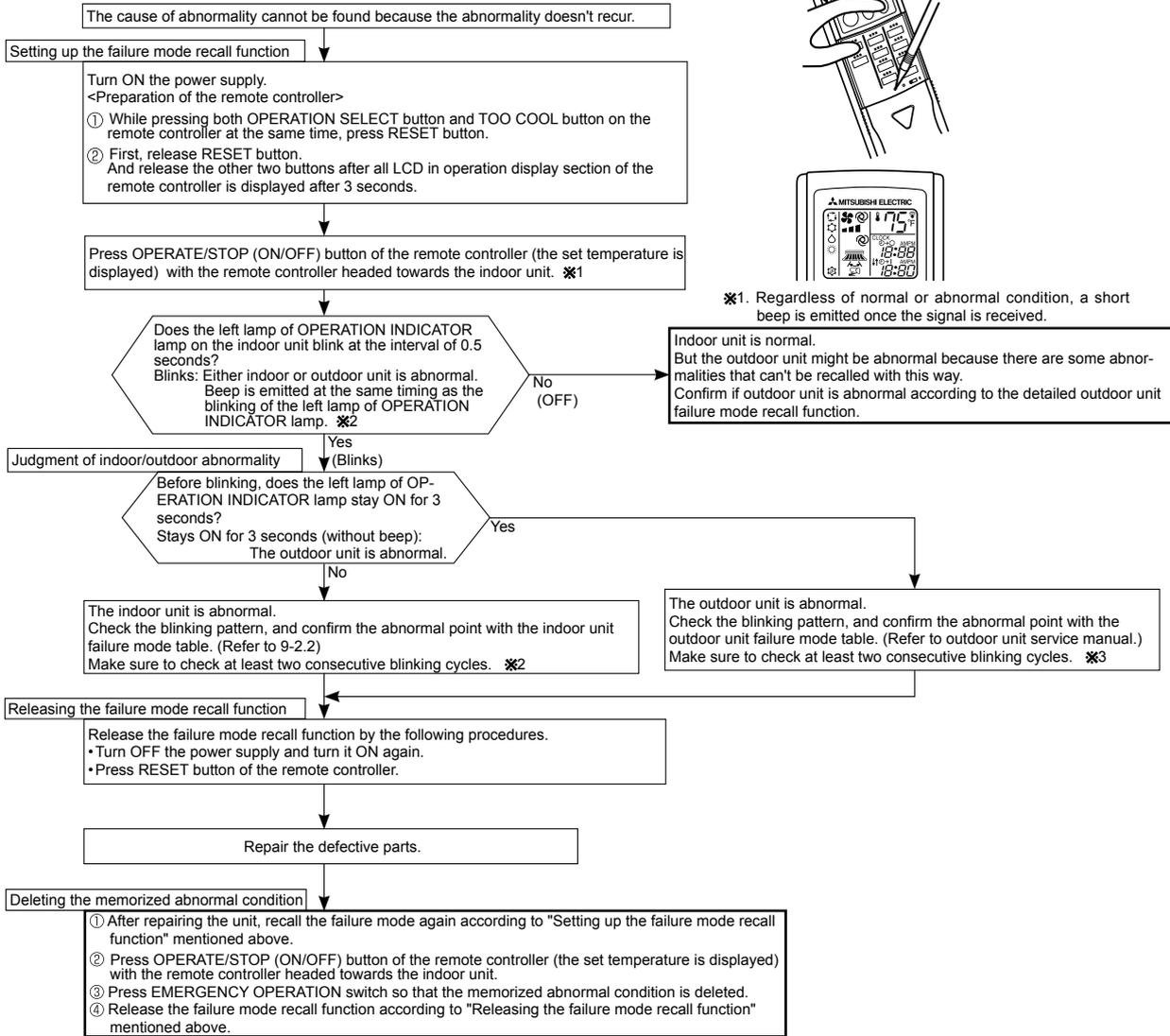
**NOTE:** 1. Make sure to release the failure mode recall function once it's set up, otherwise the unit cannot operate properly.
