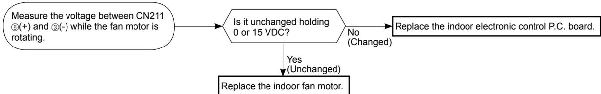
Indoor unit operates by pressing EMERGENCY OPERATION switch, but does not operate with the remote controller.
