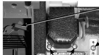
Crank of the vertical vane motor unit
