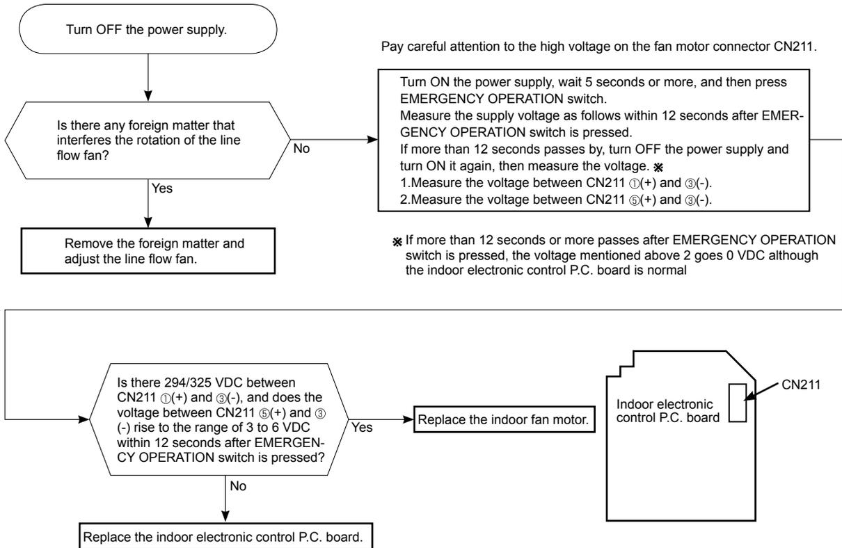
The indoor fan motor error has occurred, and the indoor fan repeats "12-second ON and 30-second OFF" 3 times, and then stops.
