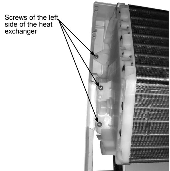
Screws of the left side of the heat exchanger
