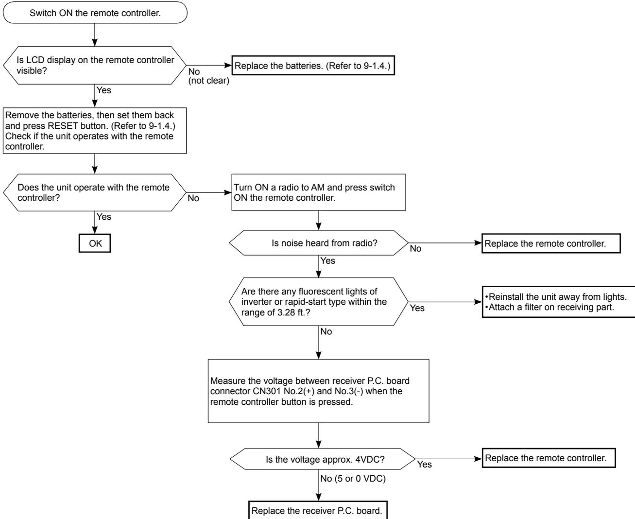
The unit does not operate with the remote controller.
