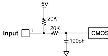
**Direction:** When this input is not active, the motor will be moving in the clockwise or “+” direction. When this input is active, the motor will move in the counterclockwise or “-” direction. This input is not read when a software index command is given. To change direction while using the software, change the direction option there. When two motors are used, the second motor will move in the opposite direction by default.
