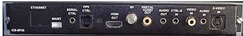
Step 4 – Attach the HDMI cable to HDMI Out on the ICS-SP30
