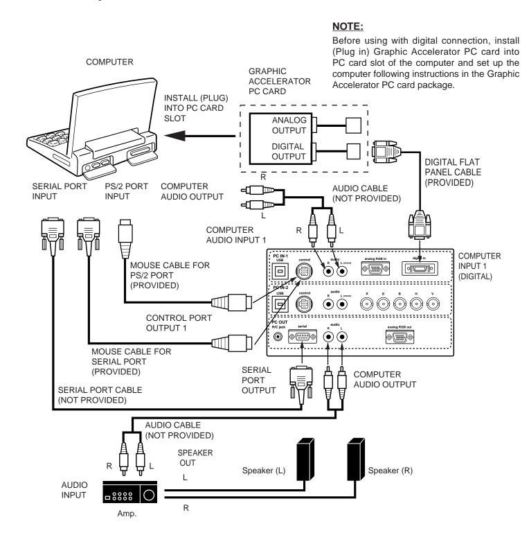
**NOTE:** The hook up should be done as per the above illustration. After hook up, turn on the projector, computer, in that order.
