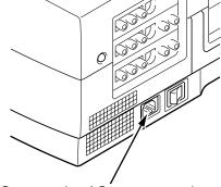
Connect the AC power supply cord (supplied) to the projector.
