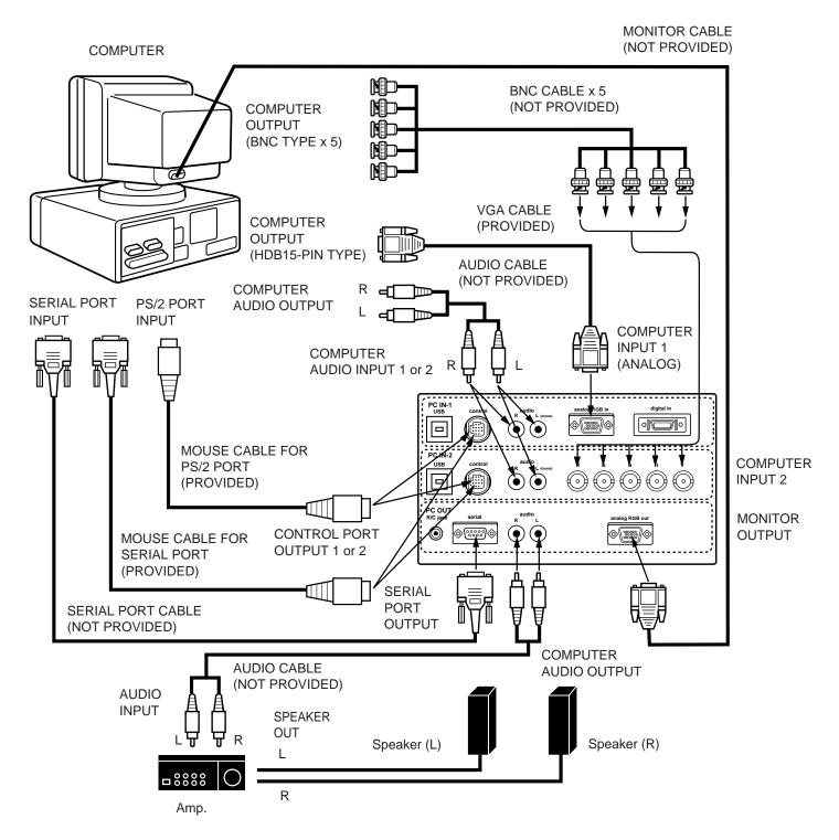
**NOTE:** The hook up should be done as per the above illustration. After hook up, turn on the projector, monitor, computer, in that order.
