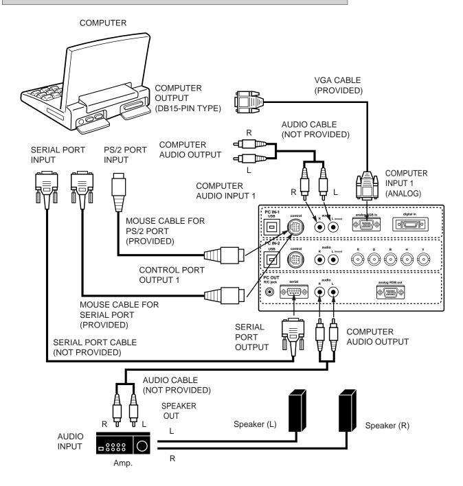
**NOTE:** The hook up should be done as per the above illustration. After hook up, turn on the projector, computer, in that order.
