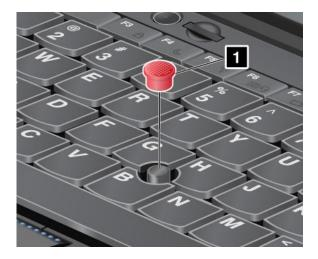
**Note:** If you replace the keyboard, a new keyboard is shipped with the default cap. If you wish, you can keep the cap from your old keyboard and use it on the new one.
