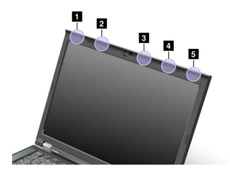
1 Wireless LAN and WiMAX combo antenna (Main)
