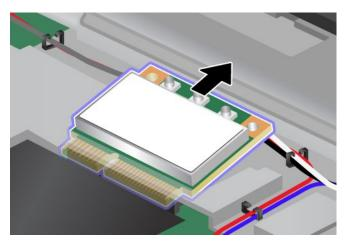
8. Align the contact edge of the new card with the corresponding socket contact of the computer 1.
