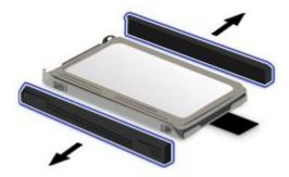
8. Attach the side rubber rails to the new hard disk drive or the side spacer rails to the new solid state drive.
