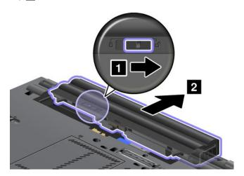
4. Install a fully charged battery until it clicks into place.
