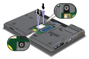
5. Put the memory slot cover back in place 1, close the cover 2, and then tighten the screws 3.
