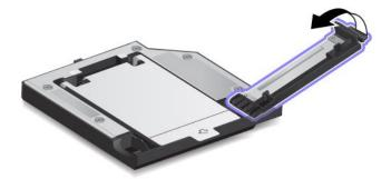
6. Insert the ThinkPad 12.7 mm Serial ATA Hard Drive Bay Adapter III into the Serial Ultrabay Enhanced bay.
