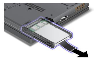
7. Detach the side rubber rails from the hard disk drive or the side spacer rails from the solid state drive.
