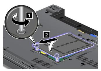
5. Remove the screws that secure the keyboard.
