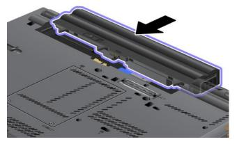
5. Slide the battery latch to the locked position.
