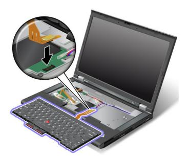
2. Insert the keyboard. Make sure that the rear edges of the keyboard are under the frame, as shown by the arrows.
