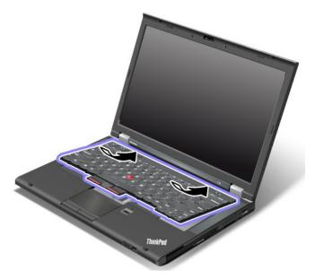
3. Slide the keyboard in the direction shown by the arrows.
