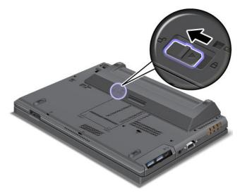
4. Press the latch as shown and detach the battery.
