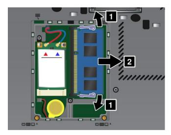
5. Find the notch on the contact edge side of the memory module you are installing.
