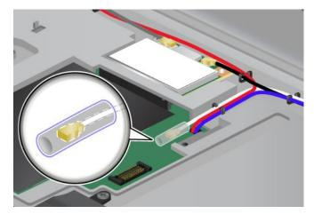
9. Pivot the card until you can snap it into place by pressing the upper side of the connectors 1. Secure the card with the screw 2.
