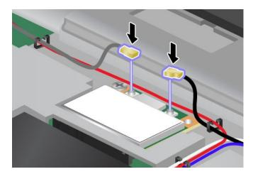
**Note:** If the new PCI Express Mini Card has three connectors, be sure to attach the gray cable to the connector marked "TR1" on the card, and the black cable to the connector marked "TR2". If you attach either cable to the center connector, the connection speed will be lower.
