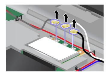
6. Remove the screw 1. The card pops up 2. Then remove the card.
