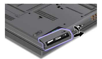
6. Remove the hard disk drive or solid state drive by pulling out the tab.
