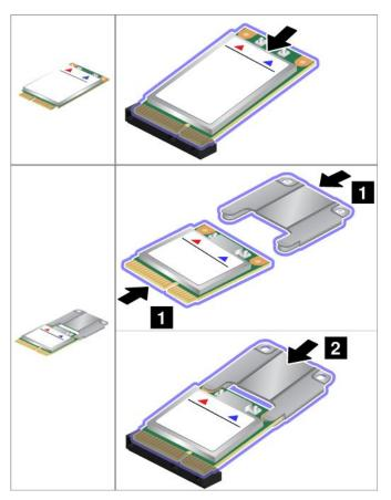
9. Pivot the card until you can snap it into place by pressing the upper side of each connector 1. Secure the card with the screw 2.
