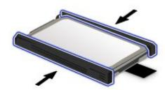
9. Insert the hard disk drive or solid state drive into the slot; then press it firmly into place.
