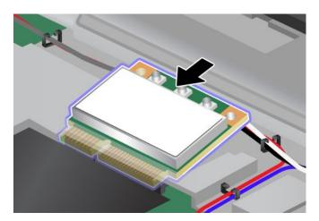
**Note:** If the new PCI Express Mini Card has two connectors, as in the next drawing, put the white cable in the cable protection tube.
