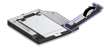
3. Insert the hard disk drive with the label facing upward.
