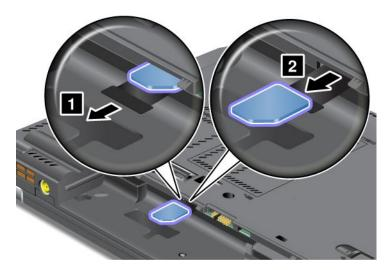
5. Hold the new card with the metal contact facing upward and going into the slot first. Then, insert the card firmly into the slot until you hear a click.
