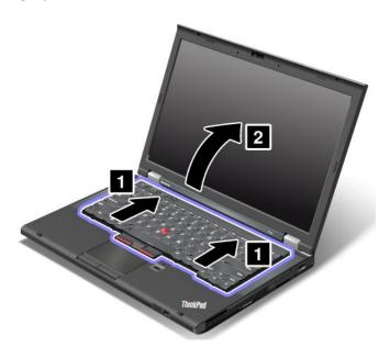
8. Carefully lift the keyboard until you can see how it is connected. Hold the keyboard above the computer, and then detach the connector 1. Remove the keyboard 2.
