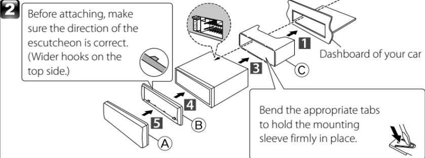
Before attaching, make sure the direction of the escutcheon is correct. (Wider hooks on the top side.)
