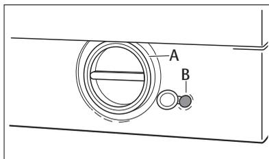
4. Release the emergency emptying hose (B), place it in the container and remove its cap cover.
