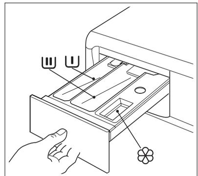
Follow the product manufacturer's recommendations on quantities to use and do not exceed the «MAX» mark in the detergent dispenser drawer. Any fabric softener or starching additives must be poured into the compartment before starting the wash programme.
