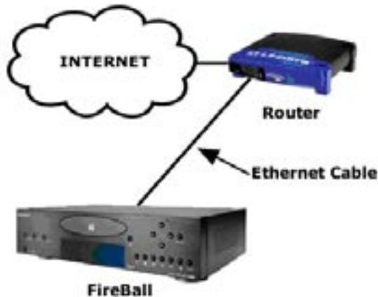
CAT5 cabling should not exceed 100 meters. The following drawing depicts the typical wiring scheme for CAT5.
