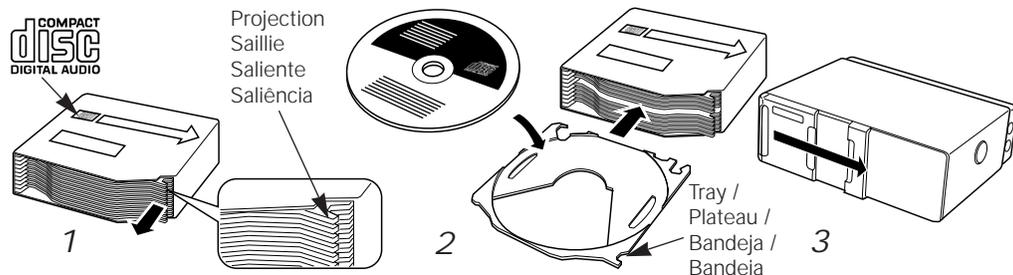
1. Make sure the disc magazine is the right way up with the "disc" logo on the top. Pull the tray out by the projection.
