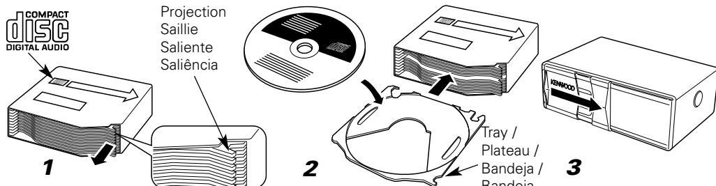
1. Make sure the disc magazine is the right way up with the "disc" logo on the top. Pull the tray out by the projection.
