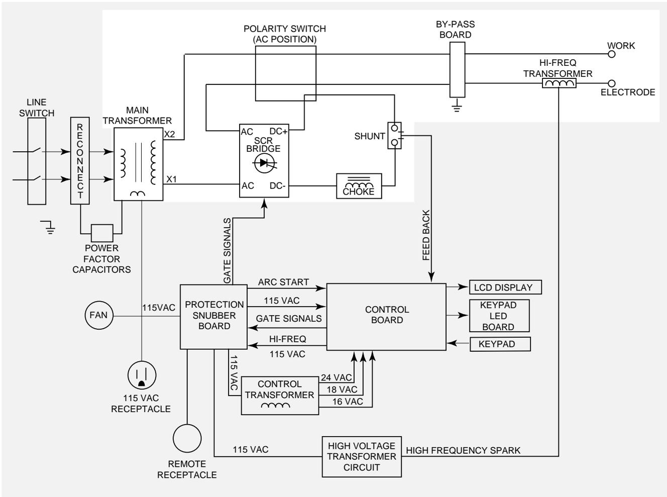
By rotating the polarity switch to the AC position the welding power circuit is changed. One lead (X2) of the main transformer secondary is connected to the machine's output work stud. The other secondary lead (X1) is connected to one of the AC connections on the SCR bridge. The electrode stud is connected
