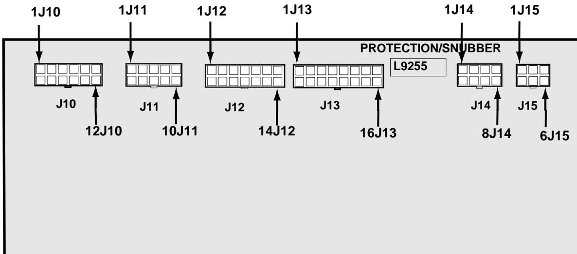
FIGURE F.6 - PROTECTION/SNUBBER BOARD TEST POINTS.
