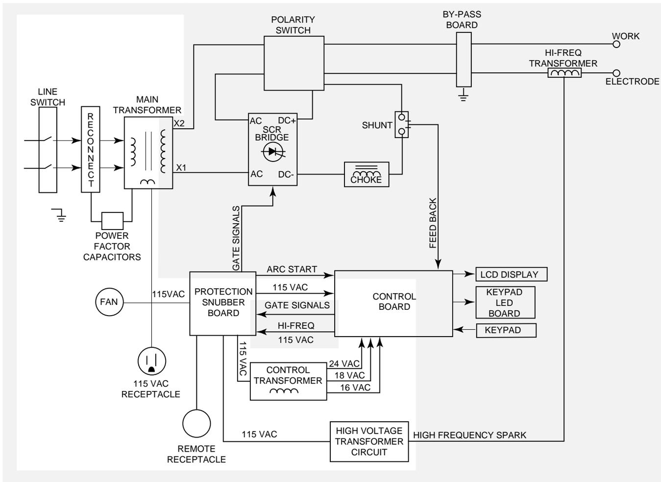
The desired single-phase input power is connected to the TIG 255 through a line switch located on the front panel.
