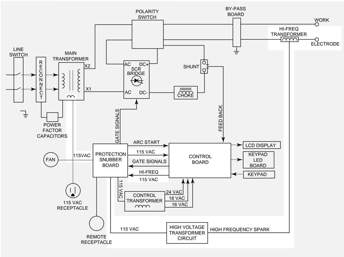
The control board passes the 115vac through the protection / snubber board to the primary of the high voltage transformer. The secondary of the high voltage transformer is coupled to a spark gap generator and also to the high frequency transformer. The high frequency transformer transfers the high frequency "spark" to the electrode stud.
