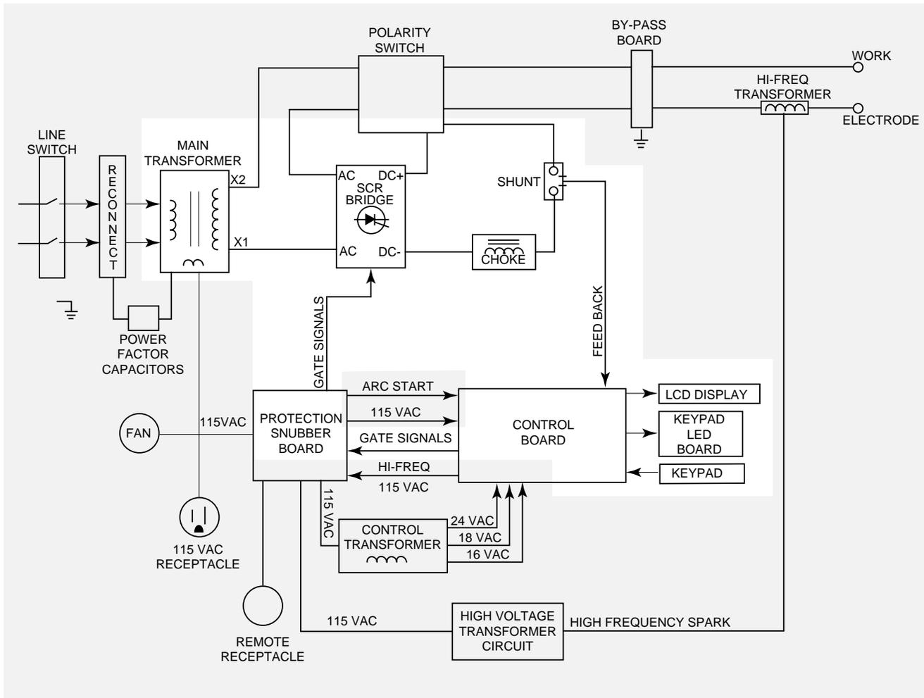
The AC output from the main transformer secondary is rectified and controlled through the SCR bridge. Output current is sensed at the shunt, as a low voltage signal, and fed back to the control board. The control board compares the commands of the keypad (or remote control) with the shunt feedback signal. The appropriate gate firing pulses are generated by
