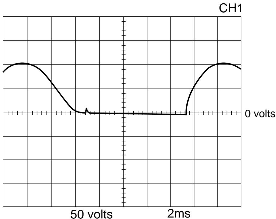
This is NOT the typical DC (+) output voltage waveform. One output SCR is not functioning. Note the “gap” in the waveform. One SCR gate was disconnected to simulate an open or non-functioning output SCR. Each vertical division represents 50 volts and each horizontal division represents 2 milliseconds in time.
