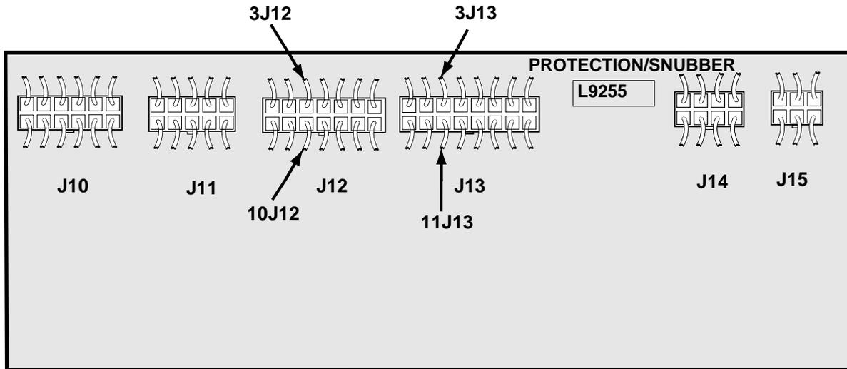
FIGURE F.9 - PROTECTION/SNUBBER BOARD TEST POINTS.
