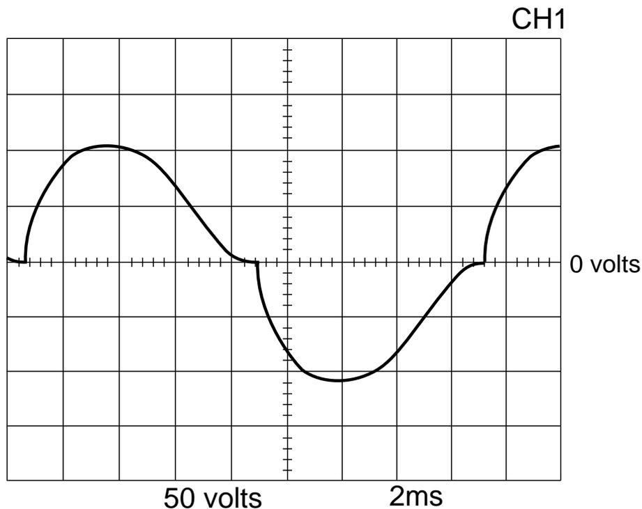
This is the typical AC output voltage waveform generated from a properly operating machine. Note that each vertical division represents 50 volts and that each horizontal division represents 2 milliseconds in time.
