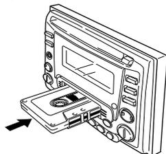
The unit turns on and tape play starts automatically. When one side of the tape reaches its end during play, the other side of the tape automatically starts playing. (Auto Reverse)
