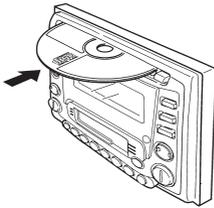
The unit turns on, draws a CD and starts playback automatically.
