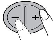
**If the input level of the external component connected to the auxiliary (AUX) input jack is not high enough, increase the input level properly.**
