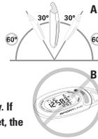
**NOTE: This Pedometer will be most accurate when worn close to the body. If the Pedometer is clipped to loose clothing or loosely contained in a pocket, the unit's accuracy may be compromised.**
