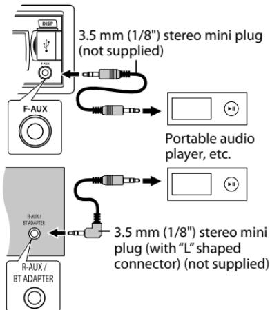
1 Connect to F-AUX on the control panel and/or R-AUX on the rear panel.
