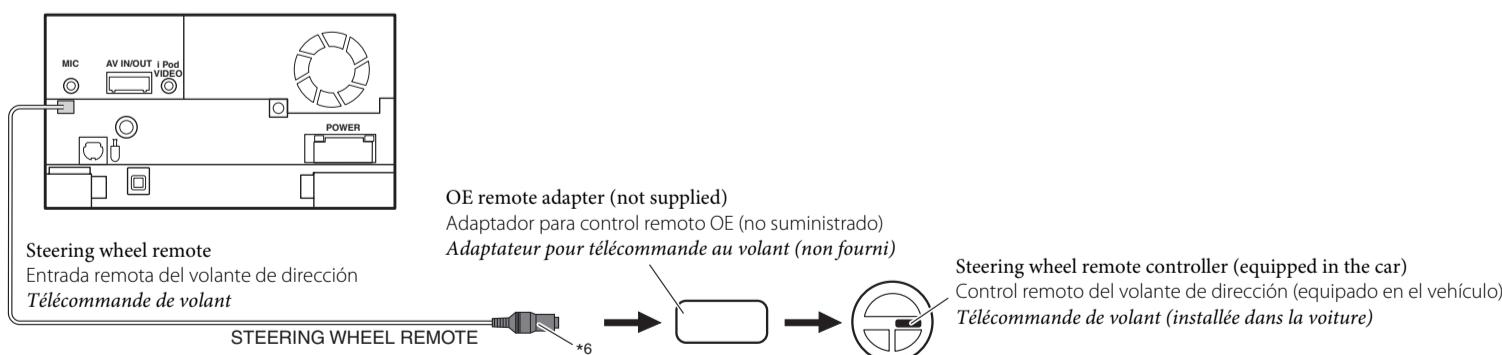
\*6 If your car is equipped with the steering wheel remote controller, you can operate this unit using the controller. For connection, an exclusive remote adapter (not supplied) which matches your car is required. For details, consult the same car audio dealer as where the unit is purchased.
