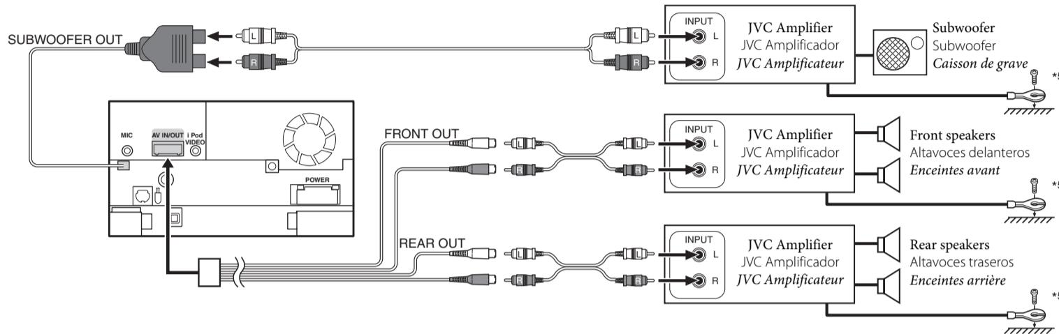
\*5 Firmly attach the ground lead to the metallic body or to the chassis of the car—to the place uncoated with paint (if coated with paint, remove the paint before attaching the lead). Failure to do so may cause damage to the unit.
