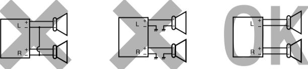
**Before connecting:** Check the wiring in the vehicle carefully. Incorrect connection may cause serious damage to this unit. The leads of the power cord and those of the connector from the car body may be different in color.
