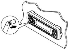
**2** Pull the control panel out of the unit.
