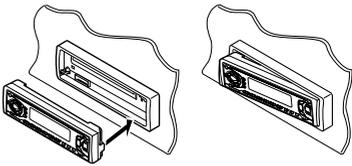
**2** Press the left side of the control panel to fix it to the panel holder.
