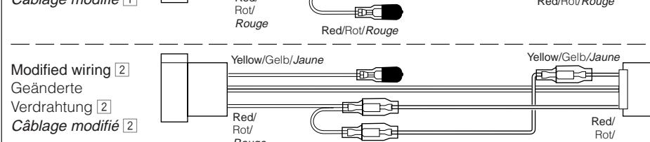
Use modified wiring 2 if the unit does not turn on.
