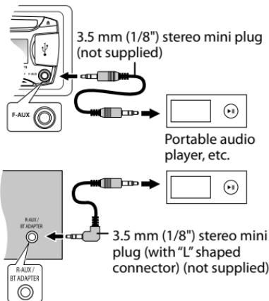
1 Connect to F-AUX on the control panel and/or R-AUX on the rear panel.
