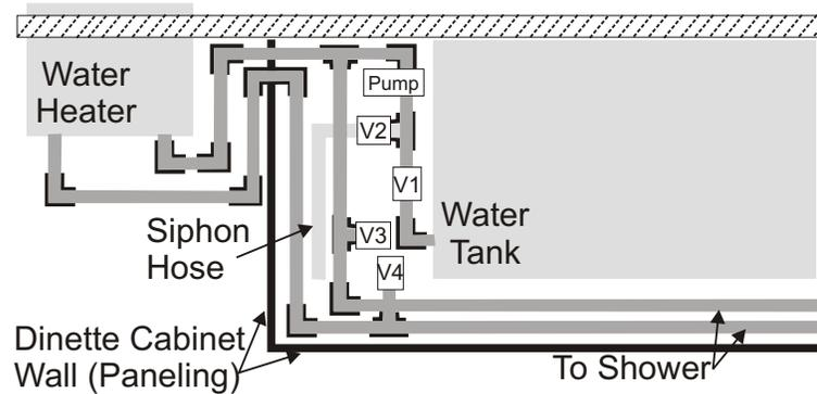
V1 = Valve that isolates water tank system
