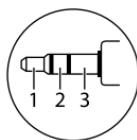
Recommended to use a 3-terminal plug head stereo mini plug for optimum audio output.
