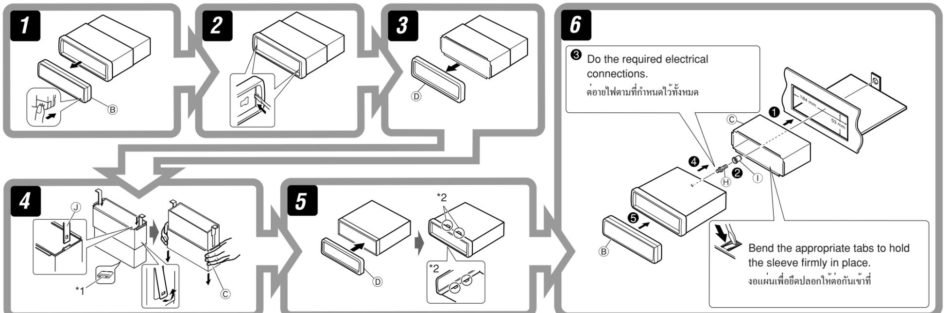
\*1 When you stand the unit, be careful not to damage the fuse on the rear.
