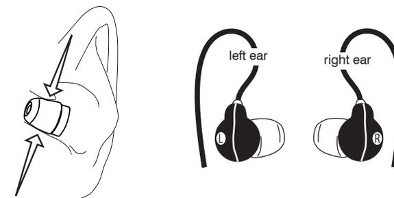
**Make sure that the sleeve completely covers the earphone stem.** If any part of the nozzle is exposed, the sleeve is not properly installed.
