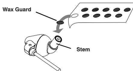
**IMPORTANT:** Do not place wax guards on sleeves! Wax guards are intended for use on the tip of the earphone nozzle only. If wax guards are placed on sleeves they will not function properly and may fall off the sleeves into your ears.
