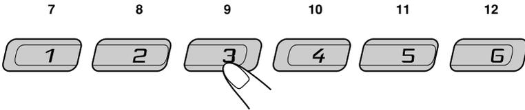
Press the number button corresponding to the disc number to start its playback (while the CD changer is playing).
