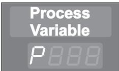
The lower display shows the output power in the form Pxxx (xxx is in the range 000% to 100% of maximum output power). This may be adjusted using the Up and Down keys.
