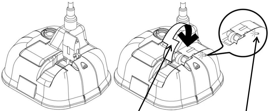
Push the main switch up 90 degrees, slide toward antenna and all the way down to activate.
