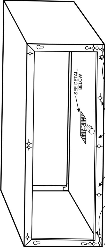
NOTE: SHADED PARTS AND SCREWS INCLUDED WITH RAD10 DRAIN KIT. THE 90° ELBOW/TUBE IS RECOMMENDED FOR INTERNAL DRAIN INSTALLATION.
