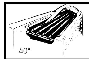
**Supply Air Throw** — One Zoneline unit should not be required to do a job obviously requiring two or more units. Units should be located around large rooms according to calculated loads or in such fashion as to achieve balanced air distribution in all parts of the room. The single unit in the "Incorrect" illustration below obviously cannot condition the entire room. Add a second unit as shown in the "Correct" illustration.
