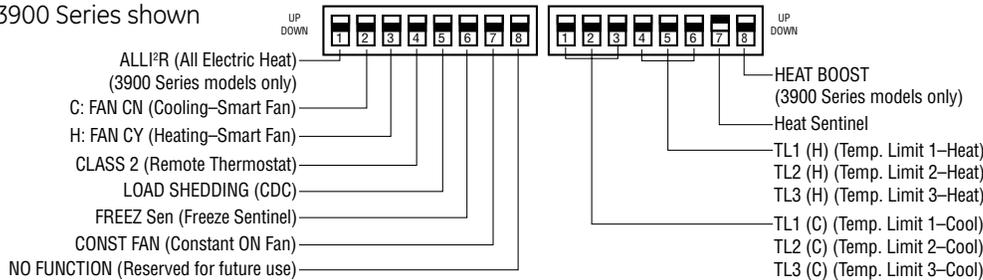
Cooling and Heating temperature limits are set independently, temperature limiting switches are in factory-set down position, except as noted.
