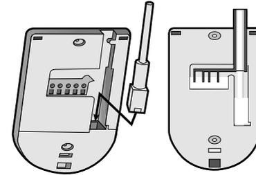
5. Align the two holes of the case-rear to the holes of the plastic anchors, and then fasten the screw-tappings (BH M3 X 30).
