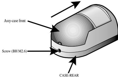
3. Place the case-rear over the installation site and mark screw holes with a pencil (indicated by the circles in the illustration). Drill a pilot hole for each pencil mark (5mm in diameter and at least 35mm in depth), and then fully insert the supplied plastic anchors (HUD 5) into them.
