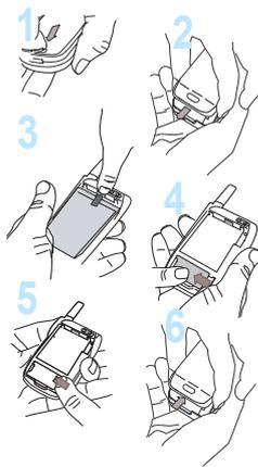
The SIM card is inserted under the phone's battery. Ensure that the phone is switched off and the charger disconnected.
