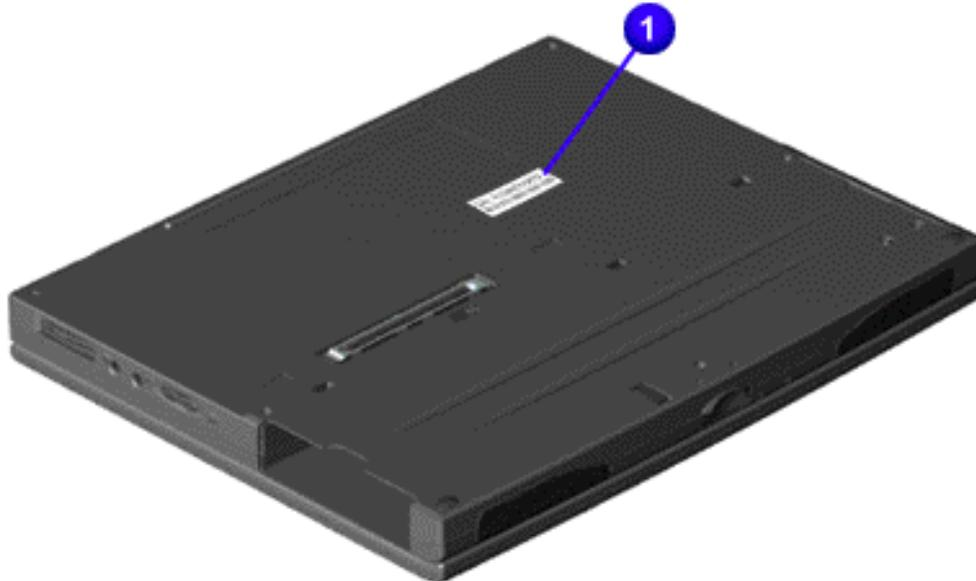
Report the computer serial number to Compaq when requesting information or ordering spare parts. The serial number is located on bottom of unit.
