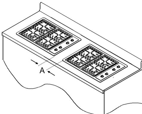
A—Minimum of 6 1/4" must separate side flanges of cooktops installed side by side.
