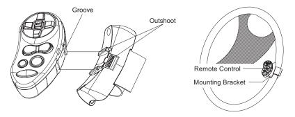
5. If the main unit is placed on the right side of the steering wheel, to operate the unit conveniently, you can install the remote control on the right pole of the steering wheel, then you can use the right hand to press the keys on the remote control to control the main unit.
