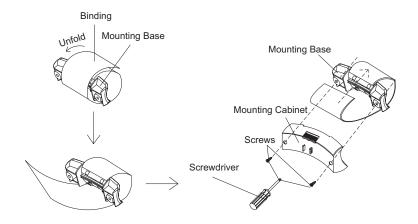
4. Fix the remote control to the mounting cabinet. Aim the outshoot on the mounting cabinet to the groove on the side of the remote control.
