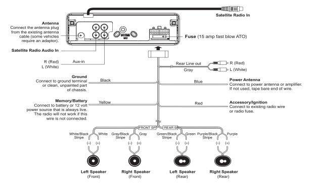
NOTE: The amplifier in this radio is only designed for use with four speakers. Never combine (bridge) outputs for use with two speakers. Never ground negative speaker leads to chassis ground. Failure to wire exactly as shown may cause electrical damage to the radio.
