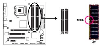
The DIMM slot has a notch, so the DIMM memory module can only fit in one direction.
