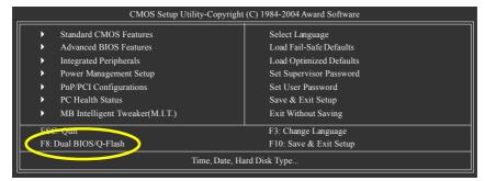
Step 2: Press F8 button on your keyboard and then Y button to enter the Dual BIOS/Q-Flash utility.
