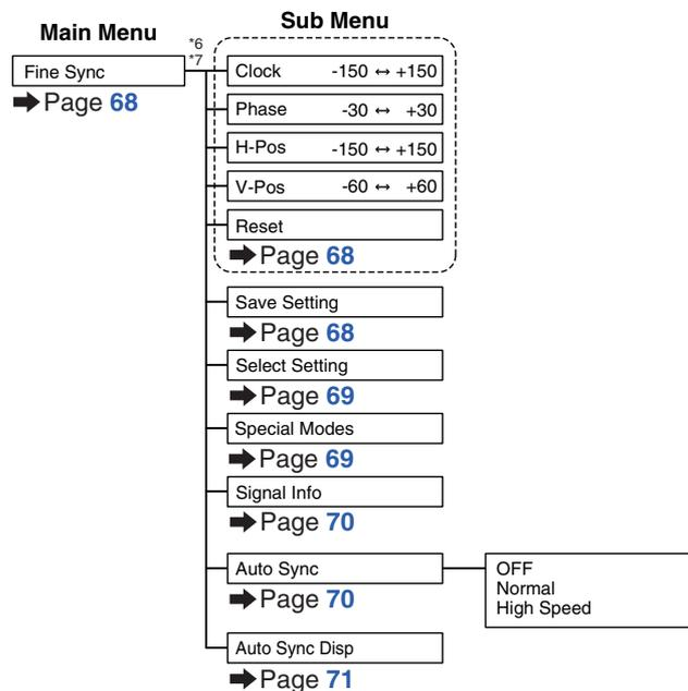
\*6 The “Fine Sync” menu is displayed only while the input mode is INPUT 1, INPUT 2 or INPUT 3.
