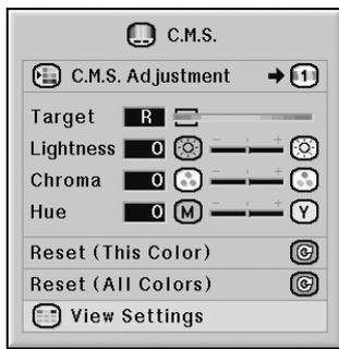
The screenshot shows the "C.M.S." screen menu. At the top, it says "C.M.S." with a printer icon. Below that is "C.M.S. Adjustment" with a right arrow and a "1" in a circle. The menu includes:
