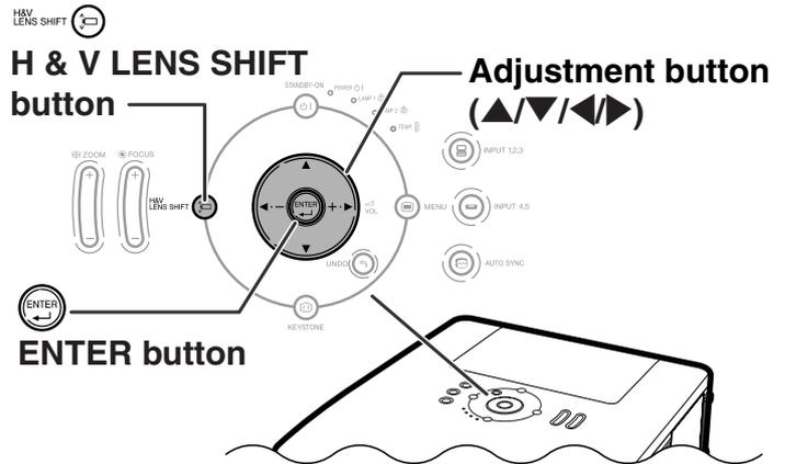
**2** Press **▲**, **▼**, **◀** or **▶** on the projector or the remote control to adjust the image position.
