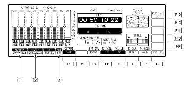
(1) **SYSTEM STATUS Display Area** Displays 2K SYSTEM mode set in SYSTEM SET UP menu.
