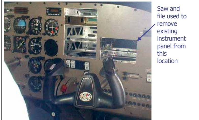
Figure 2-3 Completed panel opening (Typical)
