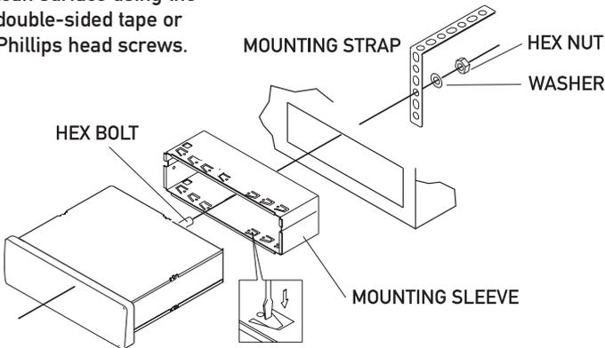
TYPICAL FRONT-LOAD DIN MOUNTING METHOD
