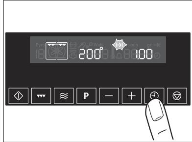
3. Using the End time
