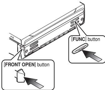
2. Deeply push in [FRONT OPEN] button to unlock the front panel.
