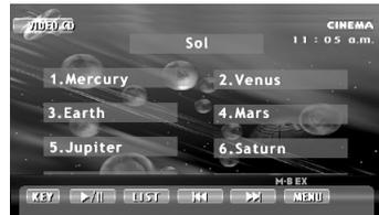
2. To select the V-CD menu contents, touch the **[KEY]** key and use either the “**Cross KEY PAD**” or the “**Ten KEY PAD**” according to the disc contents menu.
