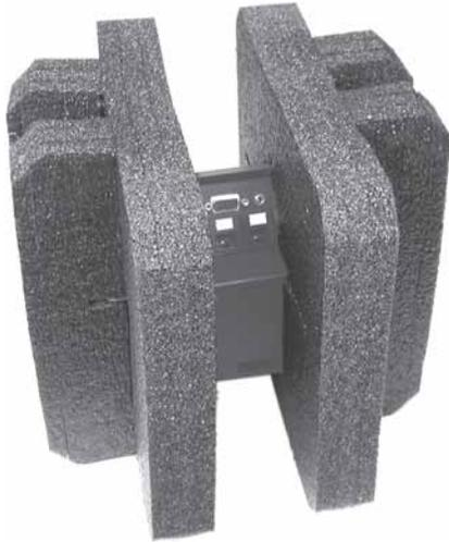
**Figure B-4 — HSA unit suspended in the foam**
